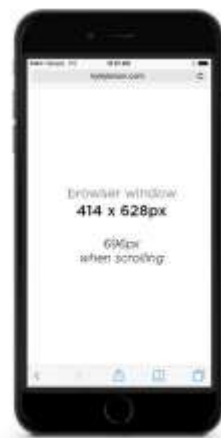
iPhone 6 Plus Display Size 5.5in Resolution 1080 x 1920px Screen Size 414 x 736px
