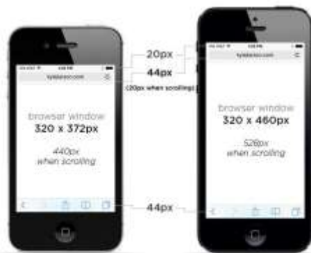
iPhone 4 (S) Display Size 3.5in Resolution 640 x 960px Screen Size 320 x 480px
